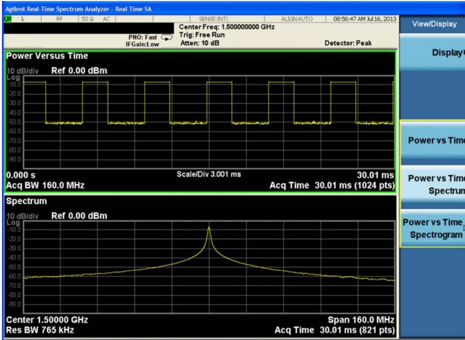
This view shows a combination of two different displays. The top window shows the Power vs. Time trace and the bottom window shows the Spectrum trace. In the bottom window, the horizontal axis represents frequency and the vertical axis represents amplitude.
