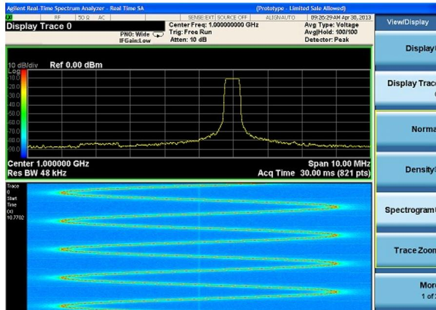
The Spectrogram View allows you to view a history of 10,000 traces, with up to 633 traces being displayed at any one time. In the Spectrogram View, each horizontal line in the spectrogram display represents one historical trace, which is the summary of an accumulation over an acquisition time interval. The data streams upwards from newest to oldest; the latest trace displays on the bottom and the oldest trace on the top.
