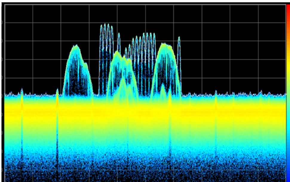
In the “**Spectrogram**” display, the same spectral data is shown with a time dimension added to the spectrum display.
