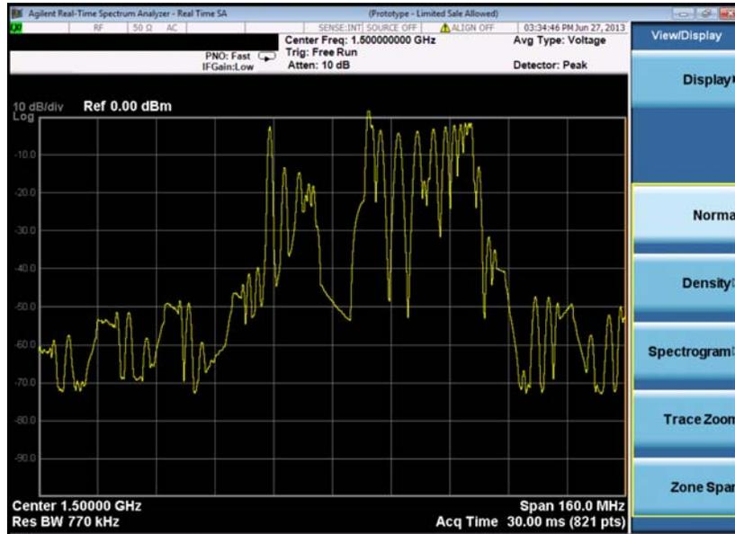
The Normal view is a single window showing Real Time, Gap Free Frequency vs. Amplitude, with frequency on the X-axis and amplitude on the Y-axis.
