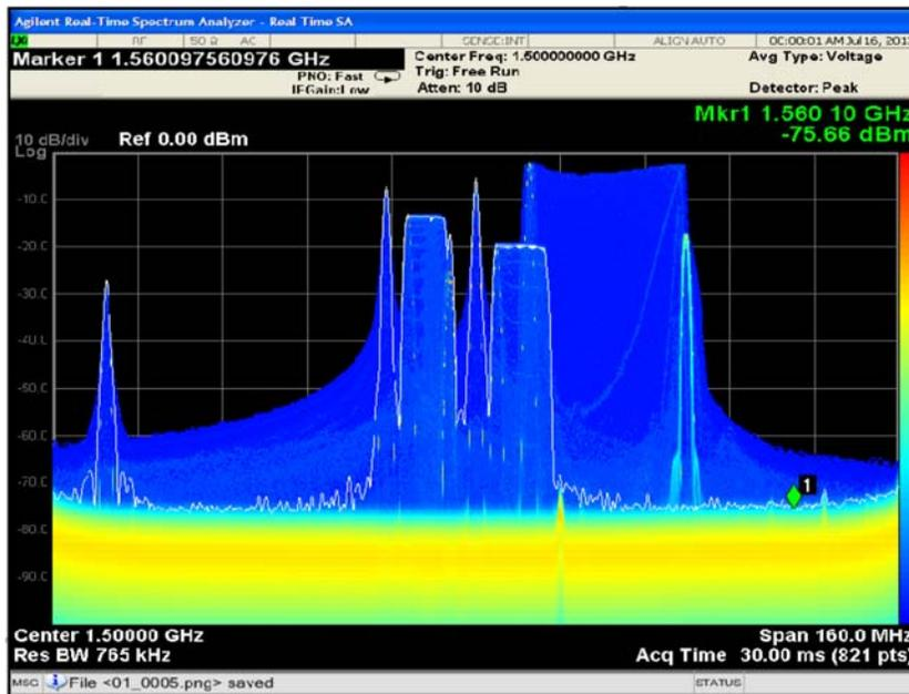
The high dynamic range enables you to see a -75 dBm signal. You can use the 89600 VSA time capture function to explore the list sweep sequence in detail.
