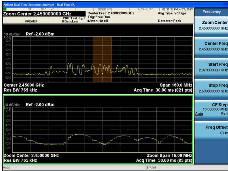
In the Trace Zoom view, the screen is split into two windows. The top window is a normal spectrum analyzer window, and the bottom window ("Zoom Window") shows a "zoomed" representation of the traces in the top window. The data in both windows is identical, but the bottom window typically shows fewer data points, spread across the whole display, which allows you to see the data in those points more clearly.
