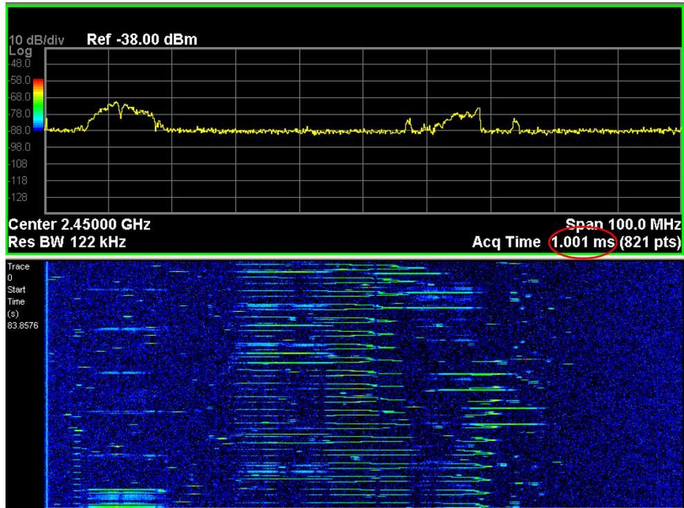
The short acquisition time can have a large effect on the appearance and content of the spectrogram display or buffer. The buffer and display will cover a proportionally shorter span of time and may not show some longer-term phenomena, but the additional time resolution can reveal important spectral behavior that would otherwise be obscured.
