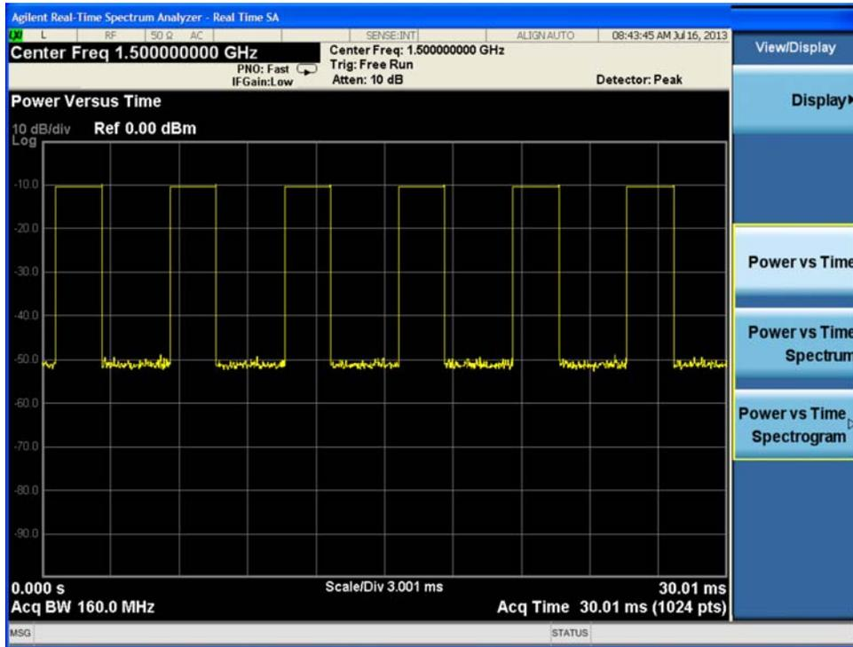
This view shows the RF envelope power over a defined time period. The horizontal axis represents time and the vertical axis represents amplitude.
