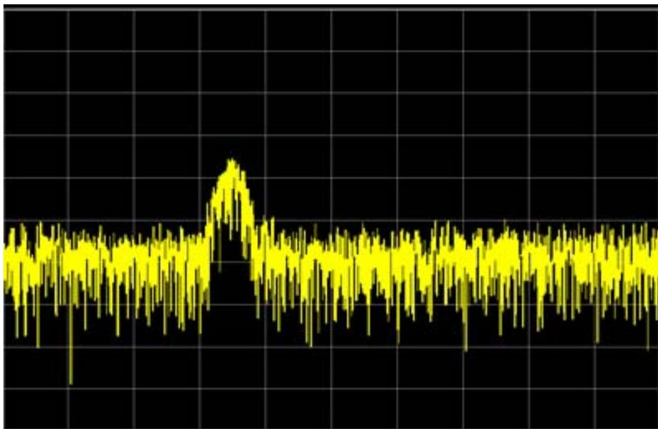
Peak hold is a useful tool for understanding some aspects of the signal environment and a long measurement with peak hold will eventually catch most of the signals in the band. However, long peak hold measurements often result in some signals in the band obscuring others. Swept spectrum analysis is not a very productive way to understand the activity in this band. Refer to the following graphic.
