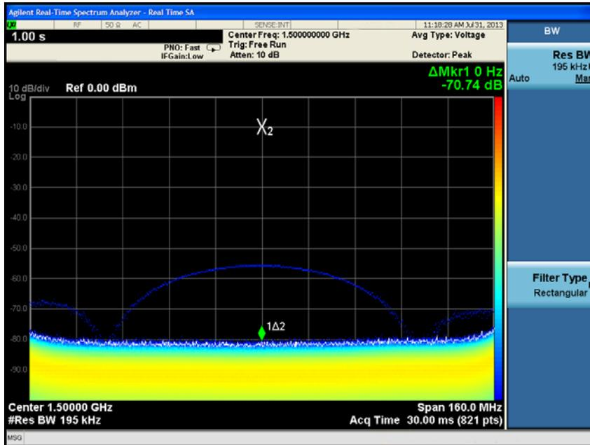
Even the narrow pulse is still captured. The Rectangular filter is used to stabilize the amplitude reading.
