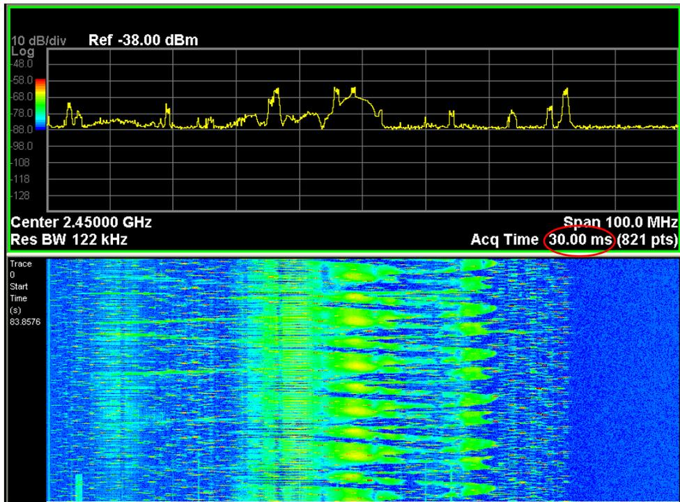
A short acquisition time has the opposite effect of the longer time of the previous example, and thus a single spectrogram display (or buffer) will represent a shorter time period, with finer time resolution.
