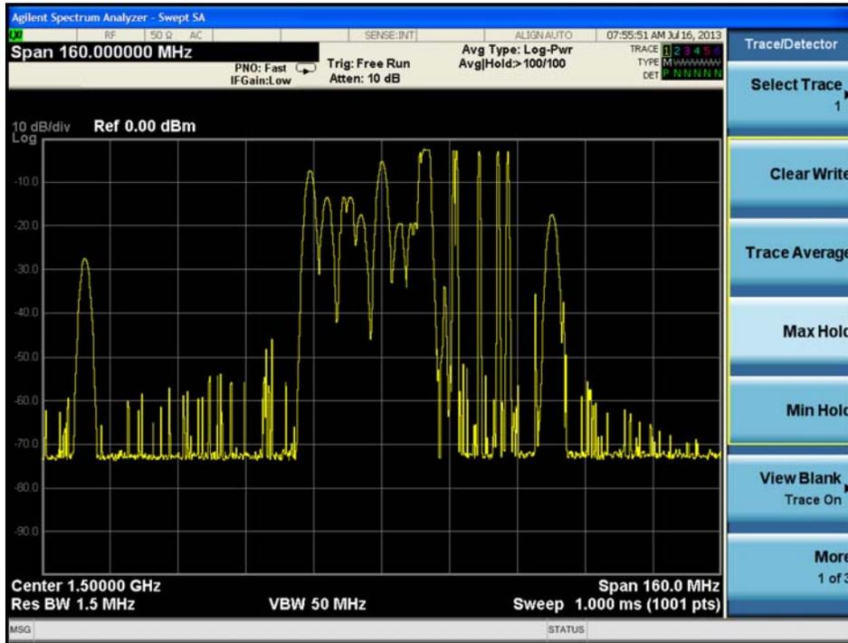
This shows a highly dynamic signal that is a challenge to view and measure. Note that in this view some signals are obscured by others.
