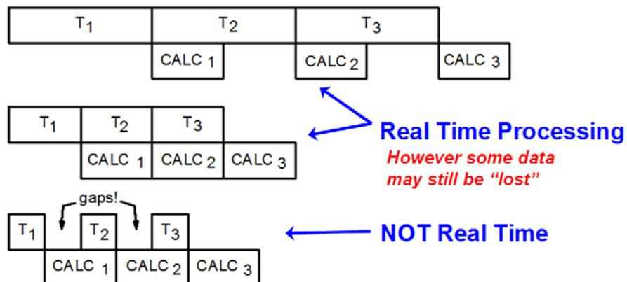
In this diagram T refers to the analyzer's time record for FFT processing. The analyzer collects a block of contiguous samples from the ADC that is digitizing the IF signal and then performs an FFT to obtain a power or vector spectrum. This sample block may vary in size or it may be fixed.
