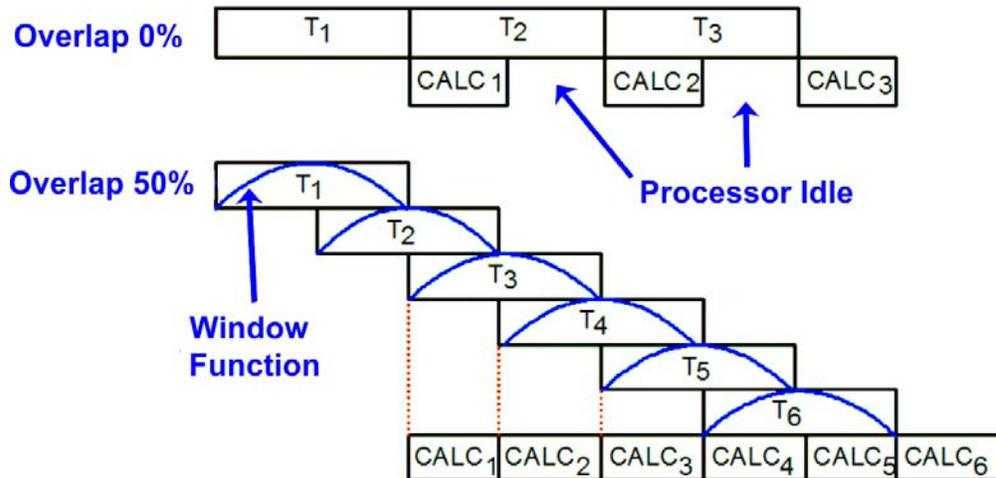
In this diagram, 50% overlap is shown, where each new FFT is performed on 50% new samples and 50% from the most recent samples of the previously processed data. Potential overlap percentages vary continuously from 0% to 100% in increments of 1 sample. Actual overlap varies depending on the analyzer and software settings, and may or may not be set-able.
