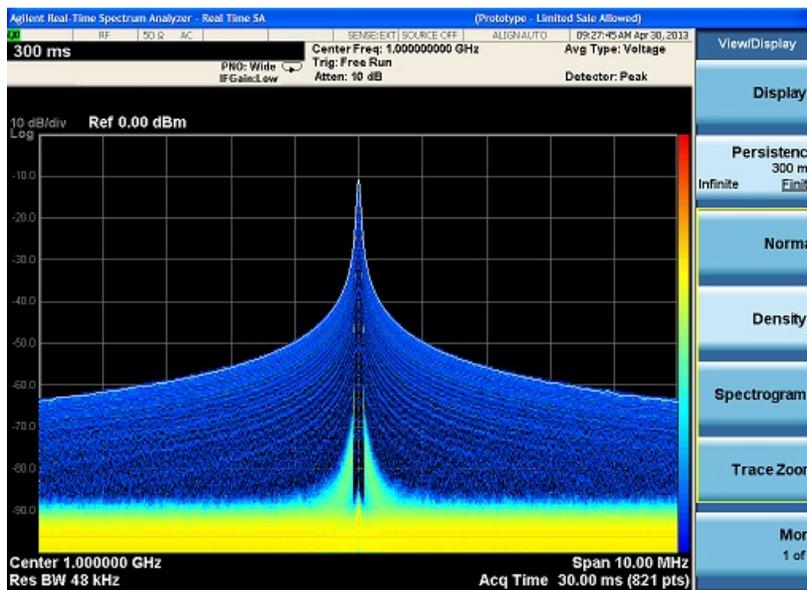
The Density view uses a bitmap to represent the signal density at each frequency and amplitude point determined by the current analyzer settings. The density is defined as the number of times a frequency and amplitude point is hit during a capture interval, which is the time a signal spends at each frequency and amplitude point in a given time period.
