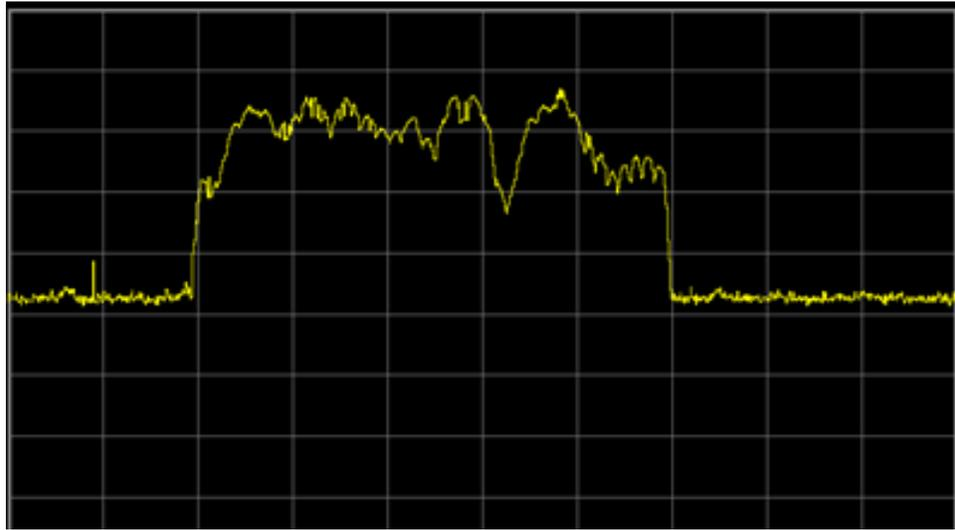
When the results are viewed in a “Density (Histogram) display, the real-time analyzer provides a good understanding of this frequency band and the signals in it. Since the measurements are gap free and all signal samples are represented in the display, it is possible to see most of the signals in the band at a glance or over a short measurement time. Individual display updates combine thousands of spectra and shows the signal dynamics and unexpected behavior.
