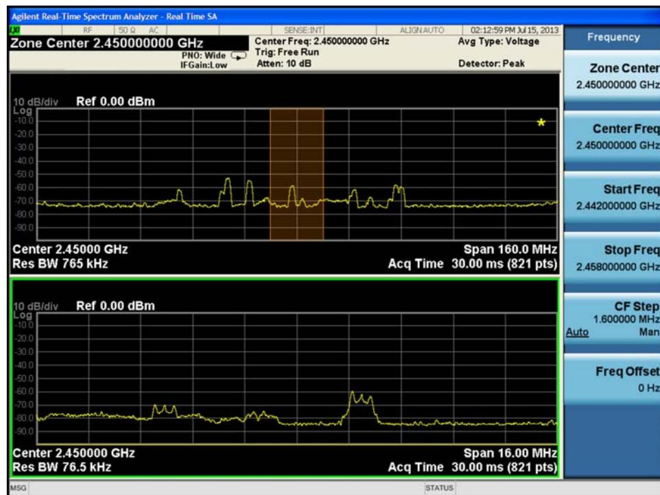
In the Zone Span view, the screen is split into two windows. The top window is a normal spectrum analyzer window, and the bottom window ("Zone Window") shows a window whose span represents a region (zone) within the top window. The data in
