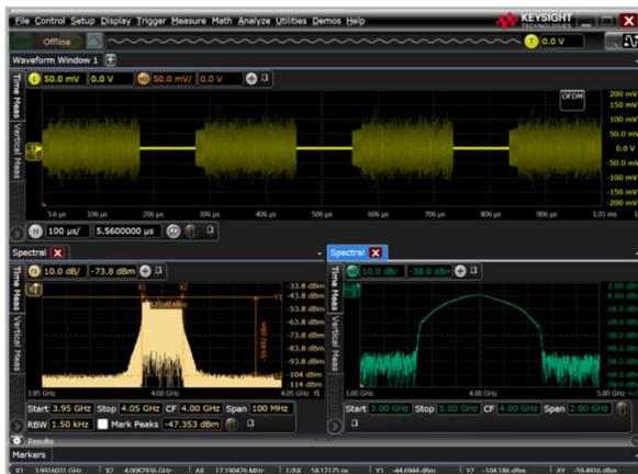
Use Infiniium capture and analysis of radar bursts as shown in this orthogonal frequency-division multiplexing (OFDM) example.
