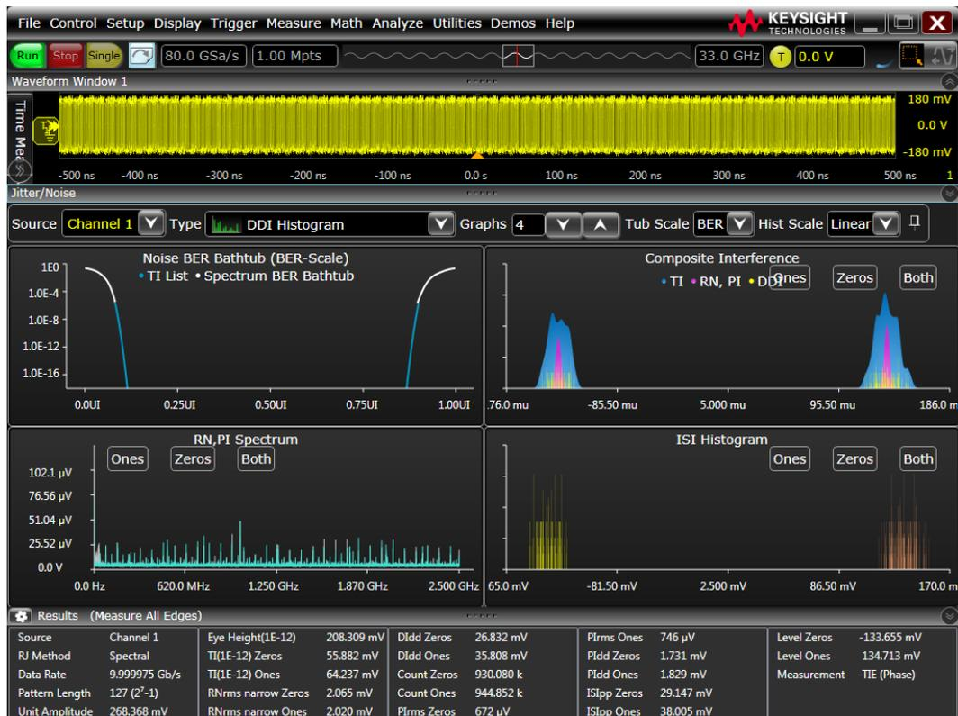
Noise analysis with EZJIT Complete software for insight into the sources of noise in the signal.
