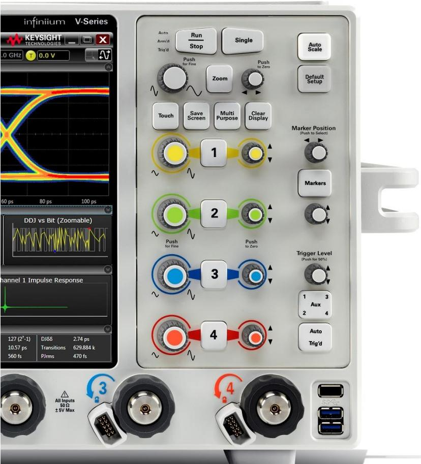
Threaded 3.5 mm RF connectors with convenient torque mechanism ensures the most reliable signal integrity and consistent 8 in. lbs. connection. The AutoProbe II interface provides a robust interface for the InfiniiMax III and III+ probing system.
