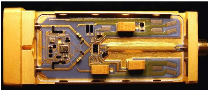
The InfiniiMax III and III+ probing system uses the same InP technology that enables high-bandwidth and low-noise oscilloscope measurements.
