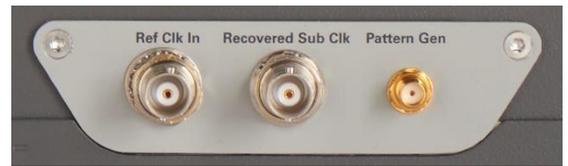
External reference clock input is one of the methods to enable SSC tracking by the hardware serial trigger.
