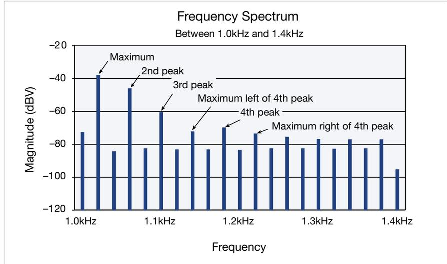
Figure 6. The 2015-P directly identifies peak values of the frequency spectrum.
