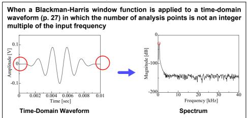
The following figure shows the time-domain waveform of the window function and its spectrum.
