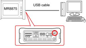
The first time you connect the instrument and PC, perform the following procedure to enable the PC to recognize the instrument.
