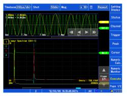
Waveform+FFT1 (Display format: [FFT])
