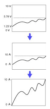
The Variable function is set as follows: Variable: On, Set Upper/Lower Limits Lower Limit: 0 [A] Upper Limit: 10 [A] The full span of output from the sensor is displayed.
