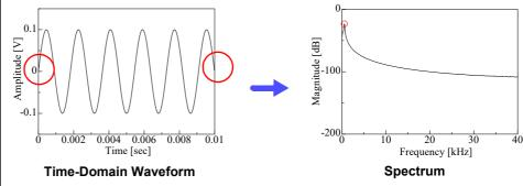
The window function was created to suppress such leakage errors. The window function smoothly connects each end of the time-domain waveform where it is cut off. The following figure presents an example of spectral analysis by applying a window function to a time-domain waveform.
