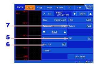
When connecting the thermocouple directly to the input module, select [Int.]. When connecting the thermocouple via a reference junction (0°C control tank, etc.), select [Ext.].
