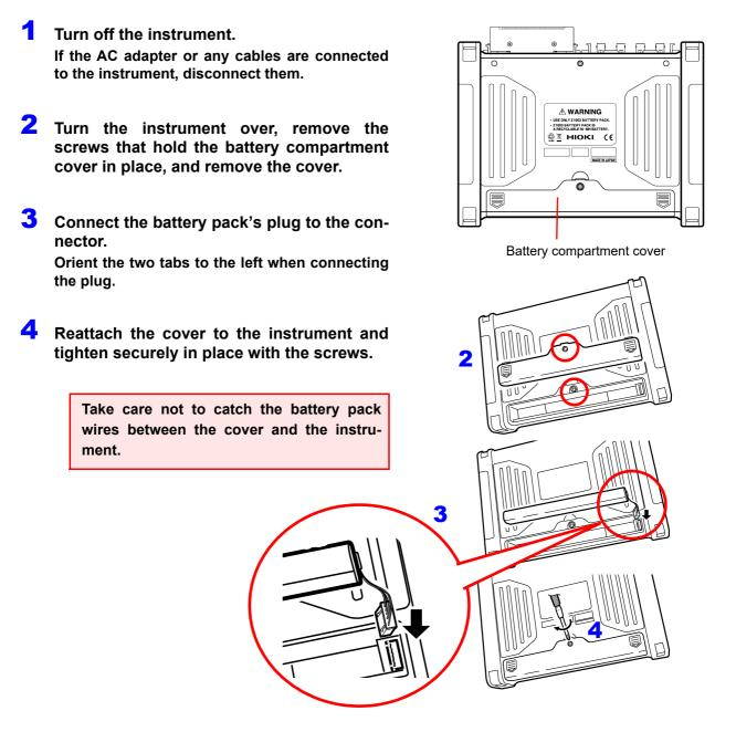
**CAUTION** Observe the correct polarity when connecting the plug to the battery pack connector. Connecting the plug with the reverse polarity could cause damage to the instrument.
