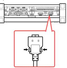
There are marks at the point at which the cable branches (CH1, CH3) (CH2, CH4). Attach sensors after checking channel numbers on the module and the marker numbers.
