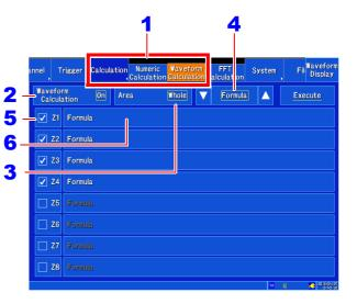
Calculation equation input formula Logarithm LOG Absolute ABS Exponer EXP Square Root SOR Derivation Integration Derivation Integration ving Ave. Cosine COS Tangent TAN SIN rallel Move SLI Arcsine ASIN Arccosine ACOS Arctangent ATAN FIR Filter FIR Filte HPFFIR FIR Filte BPFFIR FIR Filter BSFFIR Analog Channel Pulse Channe IIR Filter IIR Filte HPFIIR IIR Filte BPFIIR IIR Filte BSFIIR Channel Calc age Value Maximum Va PAVE P<u>MAX</u> Minimum Vali PMIN vel at Time PLEVEL Constant Operators
