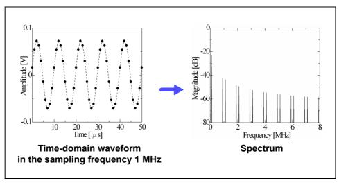
To avoid imaging phenomena when analyzing waveforms with the FFT calculation function, verify the maximum sampling frequency of the input module before measuring.
