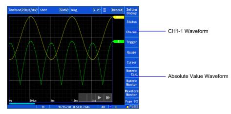
Example: Waveform of the calculated absolute value of the waveform of CH1-1. Calculation equation = ABS(CH(1,1))
