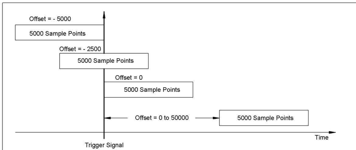
Fig. 4-5 Pre-trigger and post-trigger acquisition
