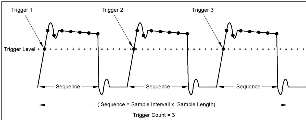
Fig. 4-6 Measurement repetition
