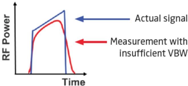
Video bandwidth (VBW) describes the ability of a power sensor to track peak (envelope) power. Insufficient VBW will result in errant envelope and average power measurements. The PMX40 offers the **widest video bandwidth (195 MHz)** making it ideal for measuring 80 MHz, 100 MHz, and 160 MHz channels.
