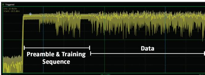
Use markers to define a portion of the waveform on which to make measurements. **“Between Marker” measurements** are ideal for monitoring specific portions of a packet over long intervals.
