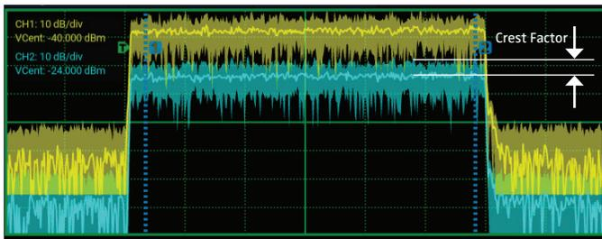
By comparing the peak-to-average power ratio, or crest factor (CF), of input and output signals of an RF transmission chain, engineers can assess circuit linearity. Additional insight can be provided with the PMX40 statistical mode **Complementary Cumulative Distribution Function (CCDF)** plot displaying the rate of occurrence of a specific CF. As an amplifier output compresses, the CF will reduce and the CCDF plot will move left.
