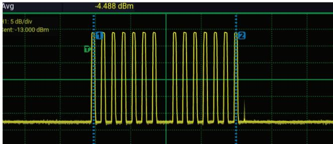
Proper design and operation of SSR systems is critical to the the safety and security of aviation. The PMX40 can be used to easily and accurately capture SSR waveforms. Markers enable measurements on specific portions of the waveform.
